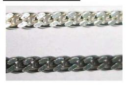
The upper chain was protected by our anti-tarnishing agent while the lower by conventional protection as known in the jewellery industry. Both chains were tested under the same conditions in 2% ammonium sulfide solution. The upper chain had no discoloration while lower chain was blackened. It proves our anti-tarnishing agent is more superior than conventional anti-tarnishing.
